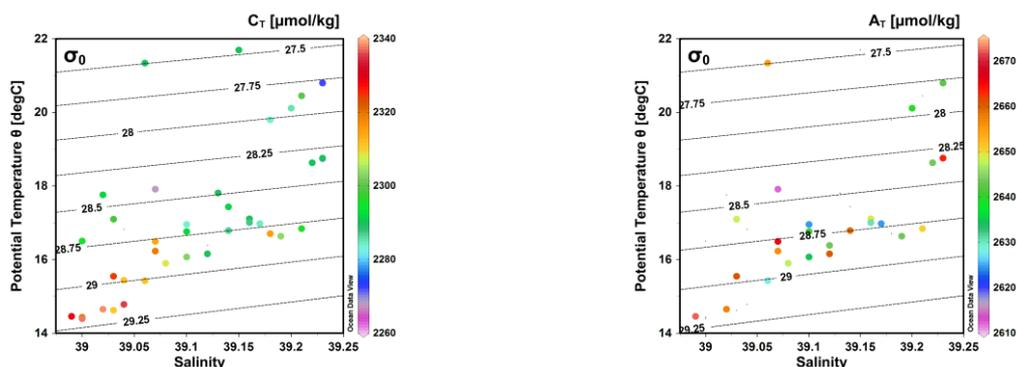
**Fig. 3.**  $C_T$  and  $A_T$  concentrations superimposed on  $\theta/S$  diagrams in Poseidon E1-M3A site during the period October 2011 to December 2013.
